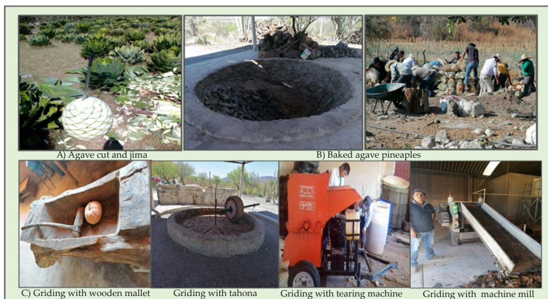
Source: prepared by the authors from survey data, 2021. Figure 2. Process of mezcal elaboration.
